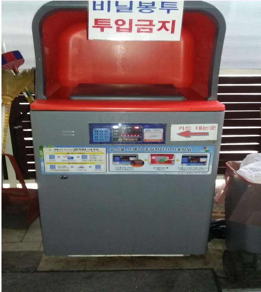
Food waste separate collection container (RFID system attached)
